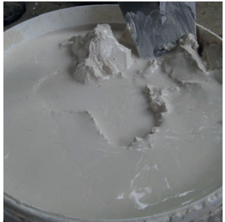
Fig. 2 Matured lime putty for use in traditional plastering can be bought from suppliers.
