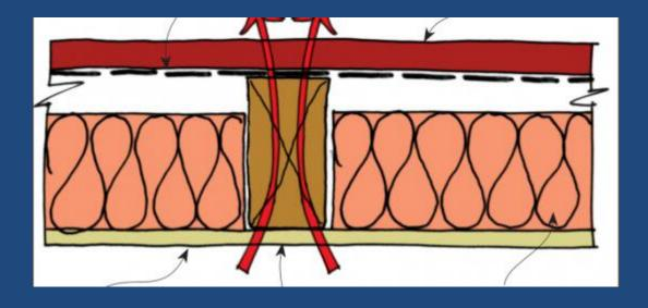
Timber joists or framing acts as a repeating thermal bridge
