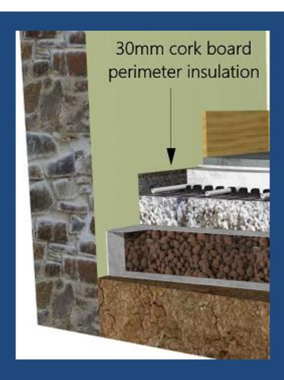
Perimeter insulation for a solid floor system reduces the heat loss into masonry – often this is omitted
